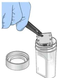
3. Lightly rinse the flow cell with laboratory-grade water, making sure that both the glass and plastic cartridge are thoroughly rinsed of excess salts.
