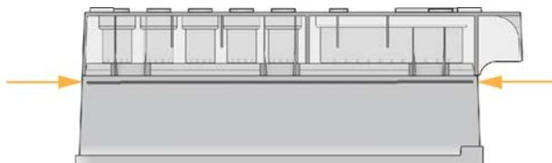
4. Allow the reagent cartridge to thaw in the room temperature water bath until it is thawed completely.
