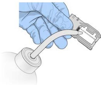
4. Using care around the black flow cell port gasket (outlined in the following illustration), thoroughly dry the flow cell and cartridge with a lint-free lens cleaning tissue. Gently pat dry in the area of the gasket and adjacent glass.
