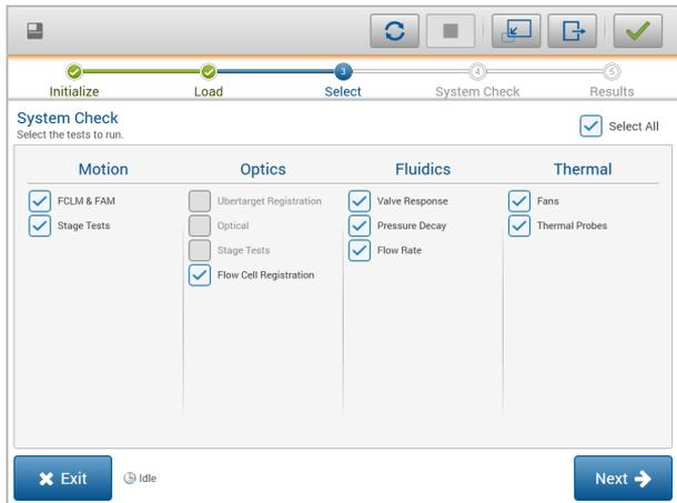
After loading consumables, the Select screen opens, which lists available system checks. Inactive checkboxes on the Select screen indicate tests that require assistance from an Illumina field representative.
