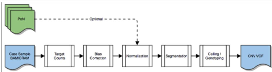
This pipeline uses many aspects of the DRAGEN platform available in other pipelines, such as hardware acceleration and efficient I/O processing. To enable CNV processing in the DRAGEN Host Software, set the `--enable-cnv` command line option to true.
