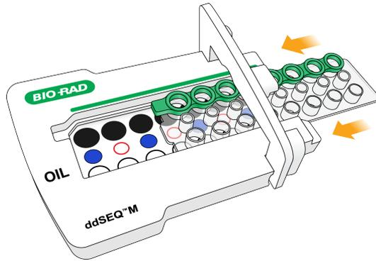
Figure 7 Incorrectly Assembled Cartridge and Cartridge Holder
