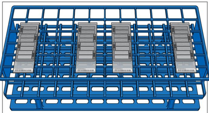
Proper BeadChip placement prevents wicking, uneven drying, and pooled dye protectant.
