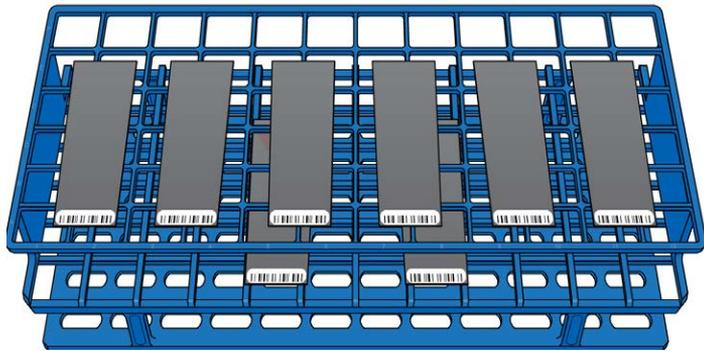
Proper BeadChip placement prevents wicking, uneven drying, and pooled dye protectant.
