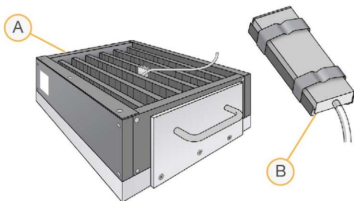
A Chamber rack with temperature probe
