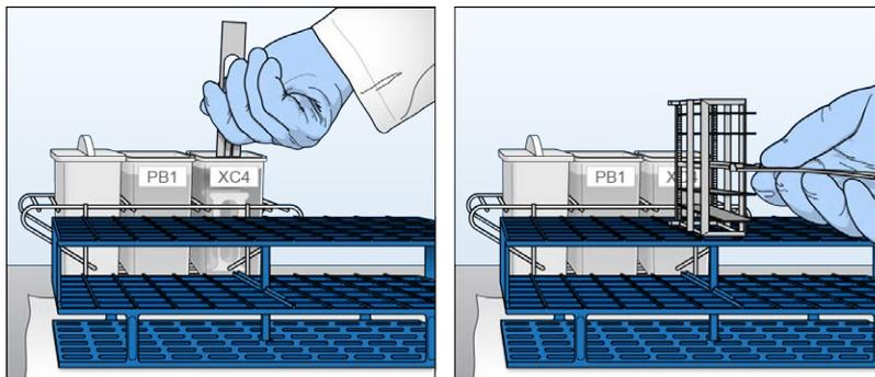
27 Make sure that the staining rack is in the center of the tube rack to ensure uniform coating. Avoid the raised edges.
