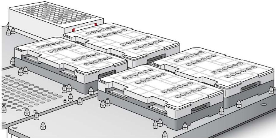
The robot dispenses sample to the BeadChips.
