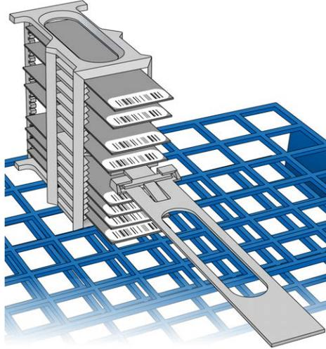
To ensure uniform coating, place the staining rack on the center of the tube rack, avoiding the raised edges.
