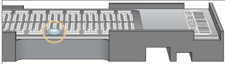
If no excess liquid is visible, it is acceptable to add additional sample from the leftover volume in the amplification plate until there is a large bolus around the loading port.
