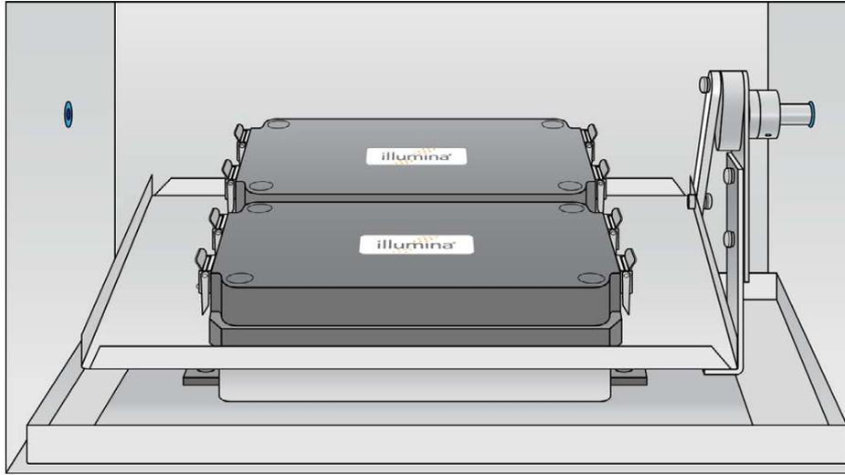
Figure 113 Incorrectly Placed Hyb Chamber
